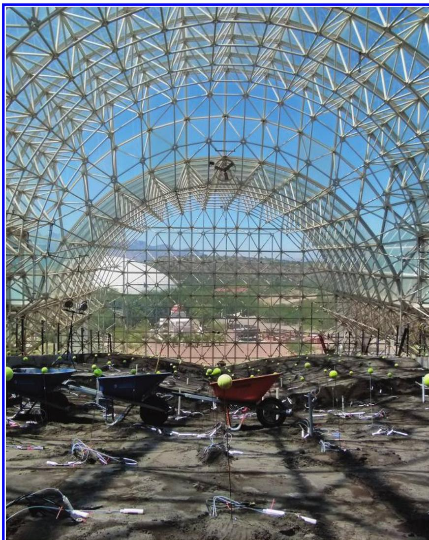
**One of the three large “landscapes” that constitute Biosphere 2’s (B2’s) Landscape Evolution Observatory. Dark volcanic soil covers the tilted platform. Sensors, their locations marked here by yellow tennis balls, will send data to B2’s computers, where researchers can control inputs (rainwater, carbon dioxide, temperature) and measure the results. Photograph: Fred Powlledge.**
